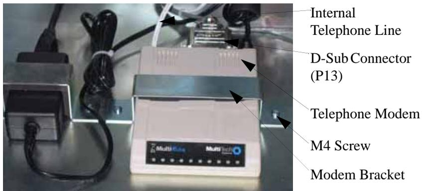
Figure 1 Installing the Telephone Modem to the GT100E
